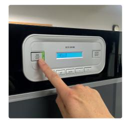
**4. Start the display** Click 'ON/OFF', green light indicates the drying cabinet is on.
