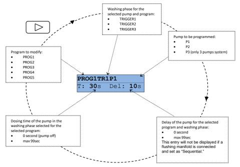
In the above example, it has been set in Schedule 1 that upon arrival of the Trigger 1, pump P1 will dose for 30 seconds, after a delay of 10 sec.
