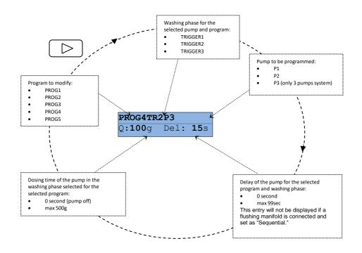
In the above example, it has been set in Program 4 that at the arrival of Trigger 2, pump P3 will dose 100g of product, after a delay of 15 sec.
