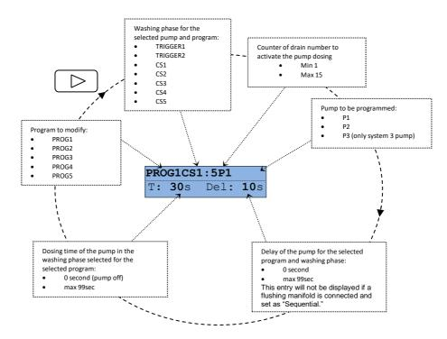
In the example above, in the Program 1, the condition CS1 is set so that once 5 drains have been counted on the input of Trigger 3, the pump P1 doses for 30 seconds, after a delay of 10 sec.
