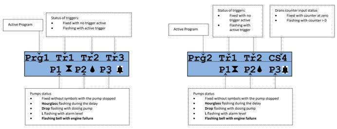
METHOD WITH TR3 (Trigger 3) SET AS DRAINS COUNTER
