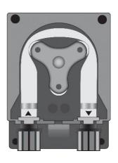
Close the pump's lid and press its surface hard so that it is properly locked into place.
