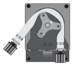
Completely release the left connector, holding it taut towards the outside, and turn the roller in the direction of the circular arrow so that the hose is freed up to the right connector.
